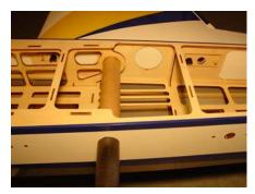
Tip#8 If the wing tube is tight you can coat the tube with a little baby powder to aid the insertion of the wing panels. However, since we now use a fiberglass insert fit should not be an issue.
