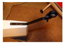
☐ Install the steel tiller horn just behind the hinge line on the bottom of the rudder using the two small wood screws.
