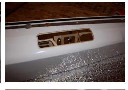
☐ Test fit the windows, as some slight trim work may be required. Once your happy with the fit, remove the protective plastic backing from the window and glue in place. We recommend glue like RC-56 as it's very strong and will dry clear
