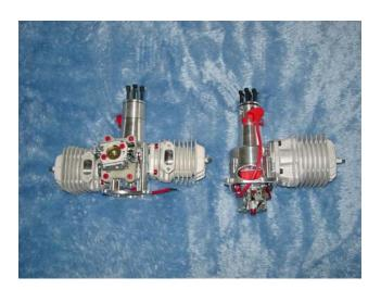
Also with the engine is installed, you will want 7-3/4 inches from the firewall to the spinner back plate for proper cowl placement.
